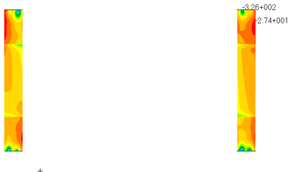
Fig 7. The Maximum Layer Stress S_{xx} in Compression in Layer Number 2 of Vertical Strut
