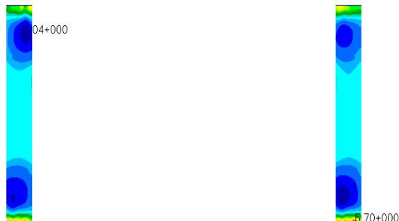
Fig 8. The Maximum Layer Stress S_{yy} in Tension in Layer Number 28 of Vertical Strut
